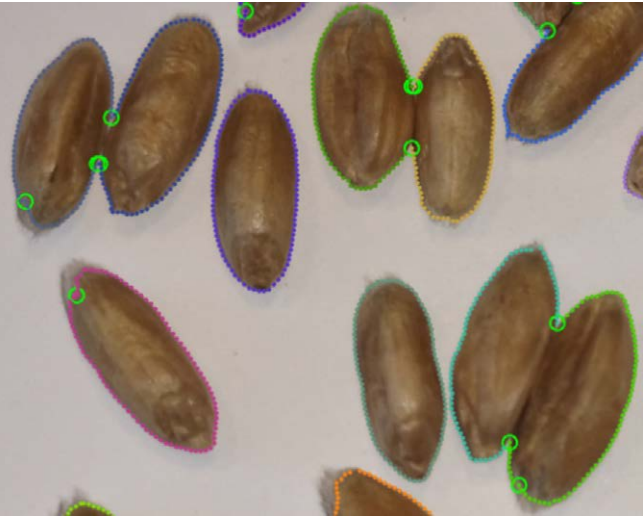
Fig. 5. The result of splitting the contours of several grain groups based on the ellipse approximation algorithm. The identified corner pixels are shown as green circles. Contour pixels that belong to the same grain are shown in the same color.
