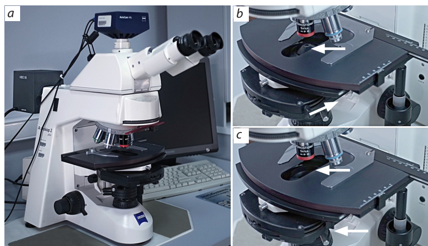
Fig. 2. Equipment for imaging: Zeiss Axioscop 2 plus microscope with an Axiocam HRC camera (2/3 inch CCD sensor) and an adapter with 0.63 magnification. Field lens 5x.
