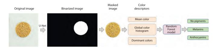
Fig. 3. Scheme of the barley grain classification model based on the Random Forest algorithm using color descriptors (the RF13 model).
