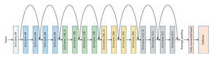
**Fig. 4.** Schematic diagram of ResNet-18 network architecture. Different-colored rectangles show network layers of different structure.
