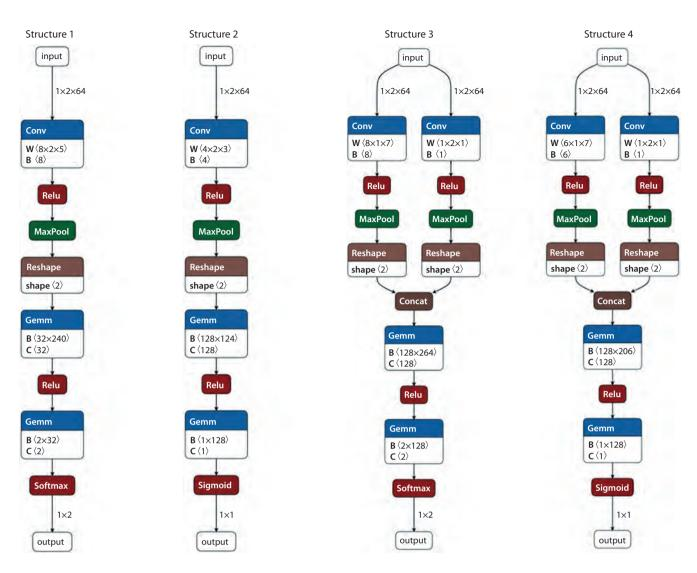
Fig. 2. Flowcharts of four models (structures) for the neural network architecture.
