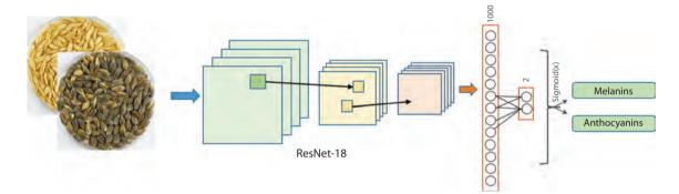
Fig. 5. Schematic of the ResNet-18 model of barley grain image classification based on convolutional neural network.
