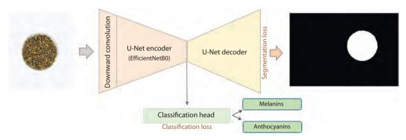
Fig. 6. Schematic of the U-Net+ClassHead model based on U-Net segmentation with a head for simultaneous segmentation and classification of barley grain images by the presence/absence of anthocyanins or melanin.
