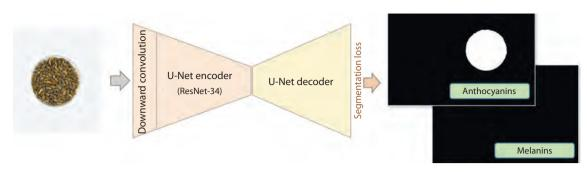
Fig. 7. Schematic of the U-Net+ClassSegment model for classification based on 2-channel segmentation of barley grain images by the presence/absence of anthocyanins or melanin.
