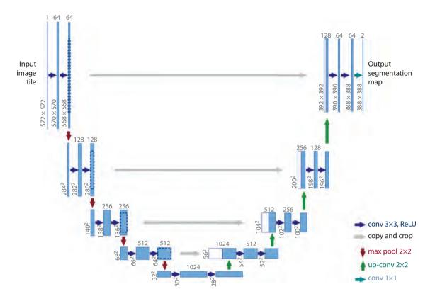
Fig. 2. U-Net network architecture used for image segmentation into grain and background regions, from (Ronneberger et al., 2015).
